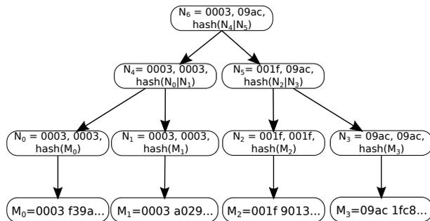
Figure 2: An example of a namespaced Merkle tree.
